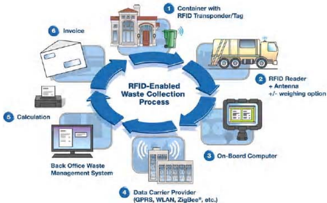
Fig. 2. RFID and Technology Enabled Waste Management Cycle (Automation of the waste collection process)
