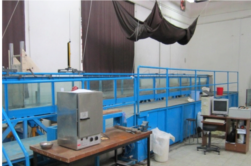
Fig. 1. A view of the flume, measurement tools, and wave-producing system
