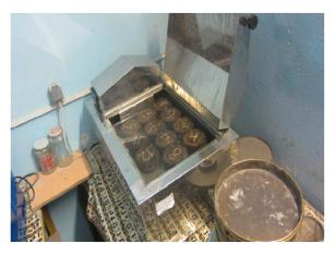
Fig. 2. Samples in the Marshall water bath
