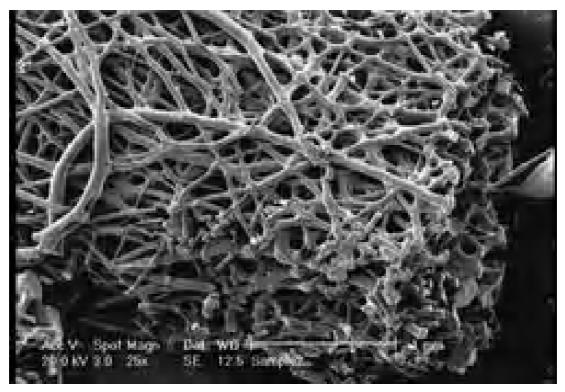
Fig. 4. SEM photo micrograph for significant effect of flow rate  $\,$  (less than 0.1 mL/min) on fiber diameter at distance between nozzle and collector of 5 cm
