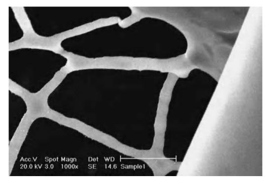
Fig. 2. SEM photo micrograph of submicron fibers produced from PET at 3 cm distance between nozzle and collector and 225  $^{\circ}$ C temperature of spinning area
