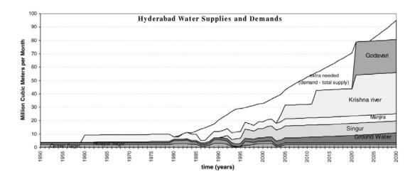
Fig. 1. Water delivery rates from the different water sources for urban water supply in Hyderabad in the period 1950–2030. For the period of 1980–2003 more detailed water delivery data were used (HMWSSB, 1995; Rooijen *et al.*, 2005)
