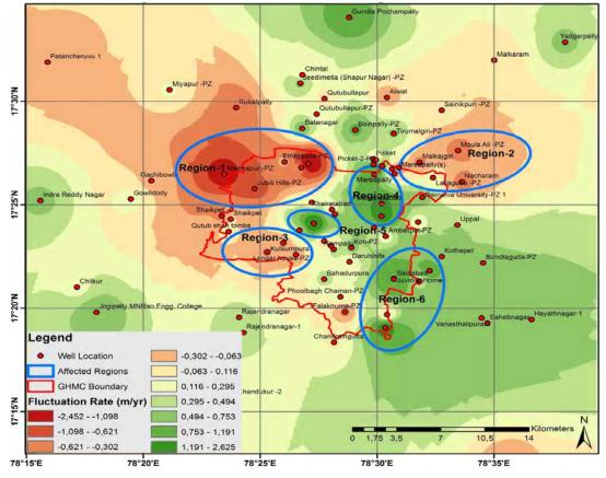
Fig. 6. Rate of groundwater table fluctuation for the period of 2003-2012 (in m/yr.)
