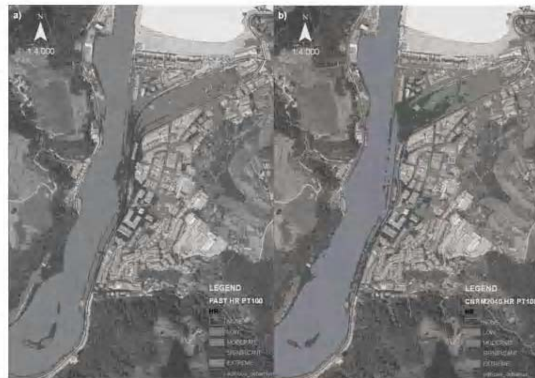
Fig. 5 a). Hazard to people data for 100 year events under past conditions (reference period, 1961-2000). b) Hazard to people data for 100 year events under future conditions (reference period, 2001-2040). CNRM model
