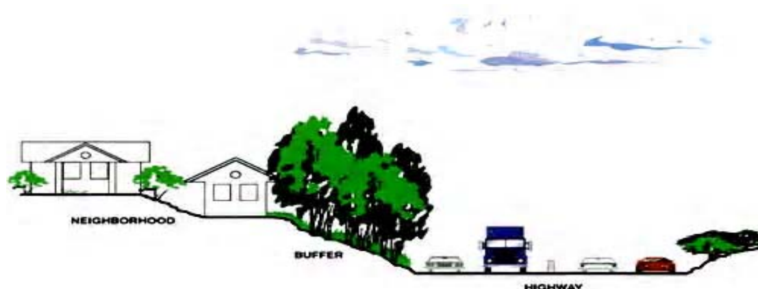
Fig. 4. Using of noise buffer zone in combination with planting vegetation in order to reduce highway noise (Center for T., 2002)
