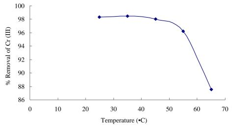
Fig. 5. Effect of temperature Cr (III) removal
