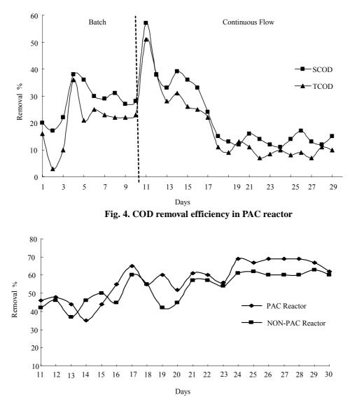
Fig. 5.  $\rm NH_4\text{-}N$  Removal in PAC and NON-PAC reactors
