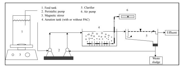
Fig. 2. Experimental setup
