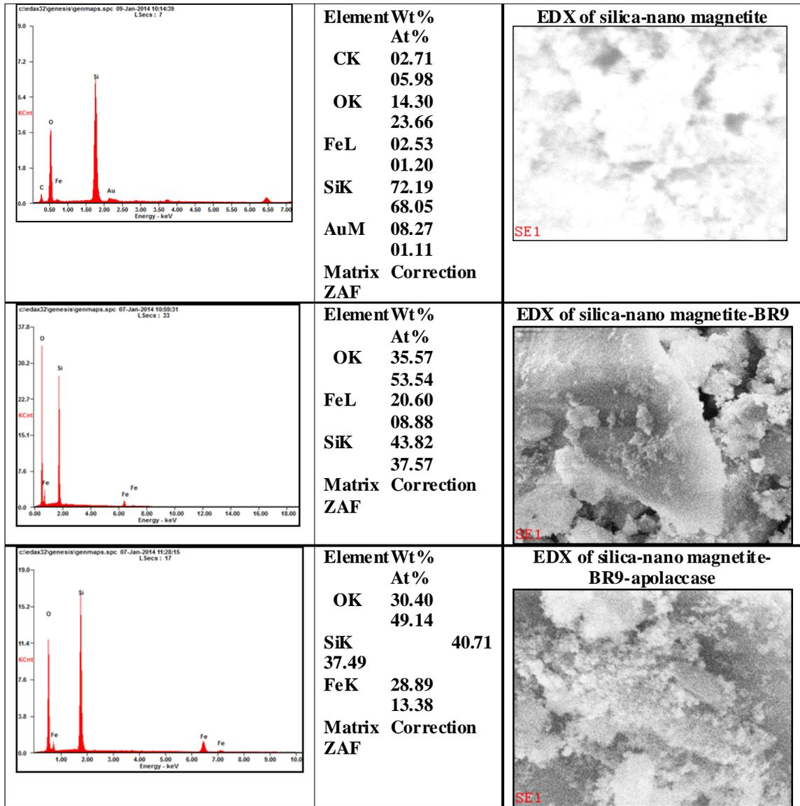
Fig. 5. EDX images of adsorbents
