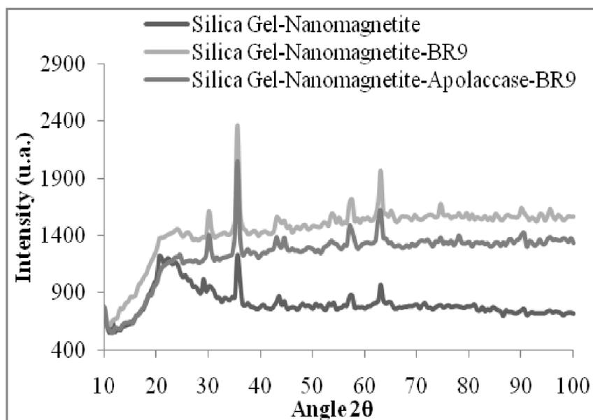
Fig. 7. XRD Images of adsorbents
