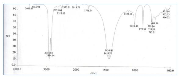
Fig. 4. FTIR spectrum of surface sterilized polyethylene treated with Alternaria alternate
