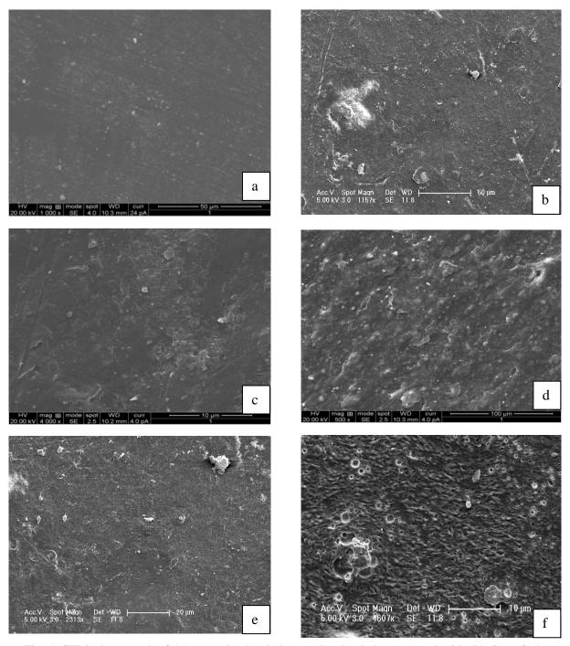
Fig. 1. SEM photograph of (a) control polyethylene and polyethylene treated with (b) *Curvularia lunata* (c) *Alternaria alternata* (d) *Penicillium simplicissimum* (e) *Fusarium* sp. and (f) consortium
