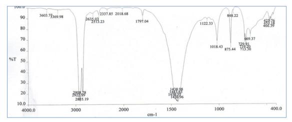
Fig. 5. FTIR spectrum of surface sterilized polyethylene treated with Penicillium simplicissimum
