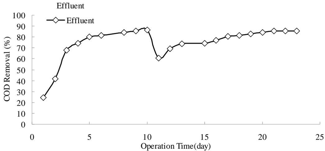
Fig.6. COD removal percentage versus operating time during the startup process of bio-trickling filter
