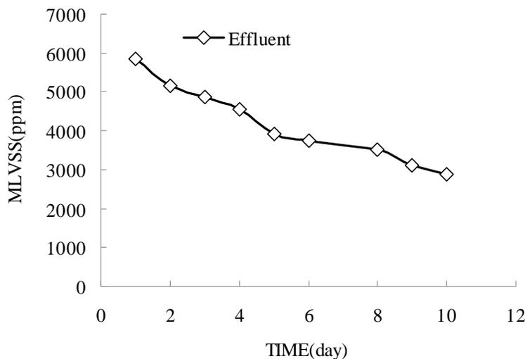
**Fig. 4. MLVSS concentration of the activated versus operating time**
