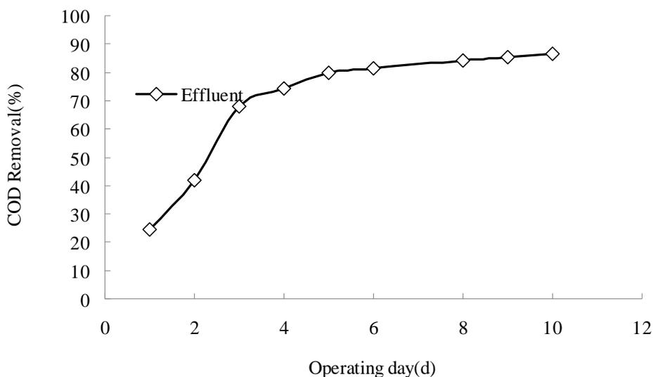
Fig. 3. COD Removal percentage of the activated sludge versus operating time
