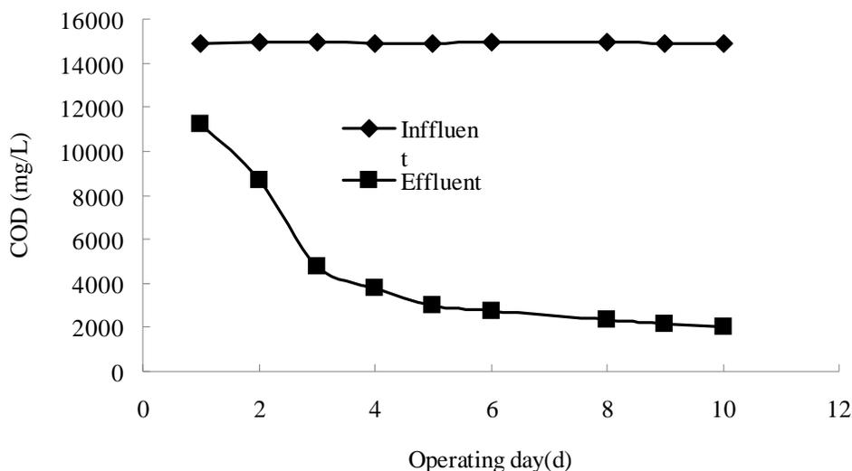
Fig. 2. COD concentrations of the activated sludge versus operating time (Q=0.0035 L/min)
