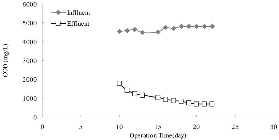
Fig.5. COD concentrations of the activated sludge with extra nutrients versus operating time ( $Q=0.0045$  L/min)
