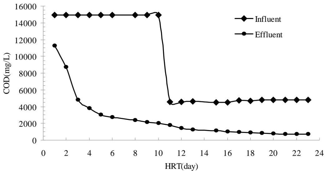
Fig. 7. COD concentration versus operating time during the startup process of bio-trickling filter
