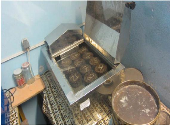
**Fig. 2. Samples in the Marshall water bath**
