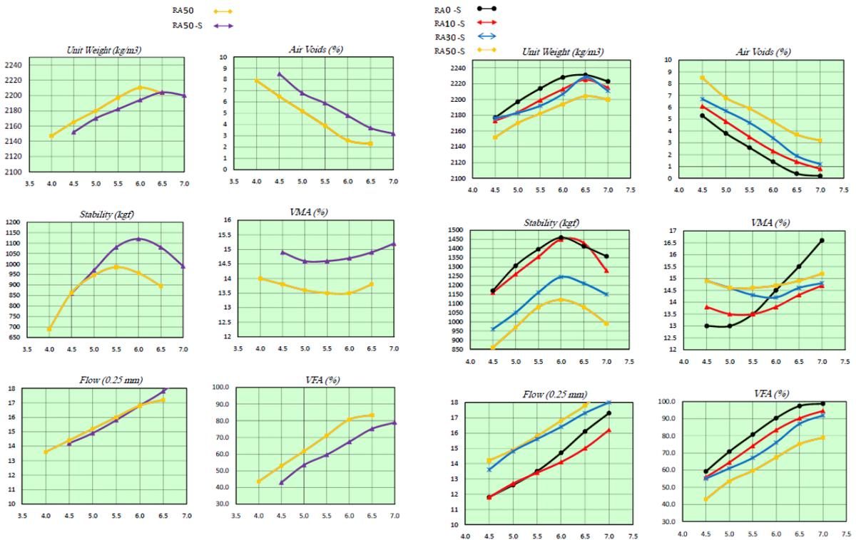
Fig. 4-A. Comparison of the physical and mechanical properties of RA50 and RA50-S mix designs
