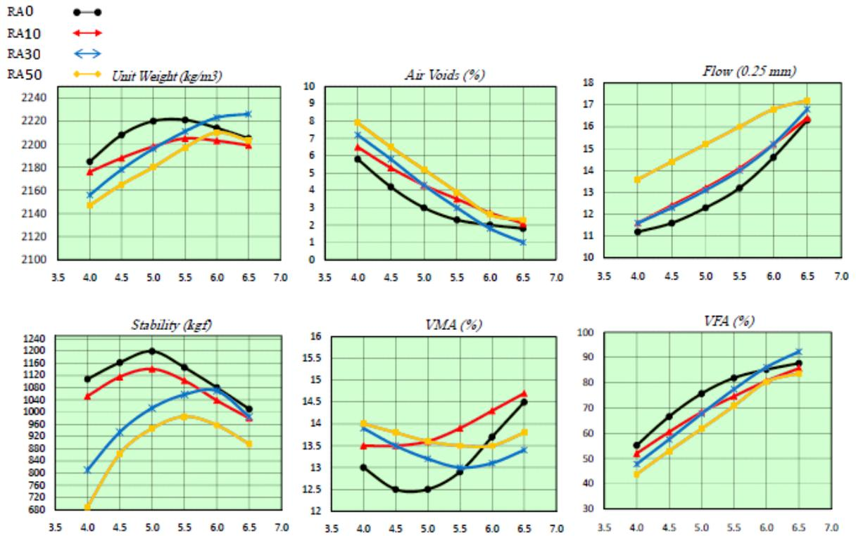
Fig. 3. Comparison of different asphalt concrete mix designs parameters obtained from Marshall test
