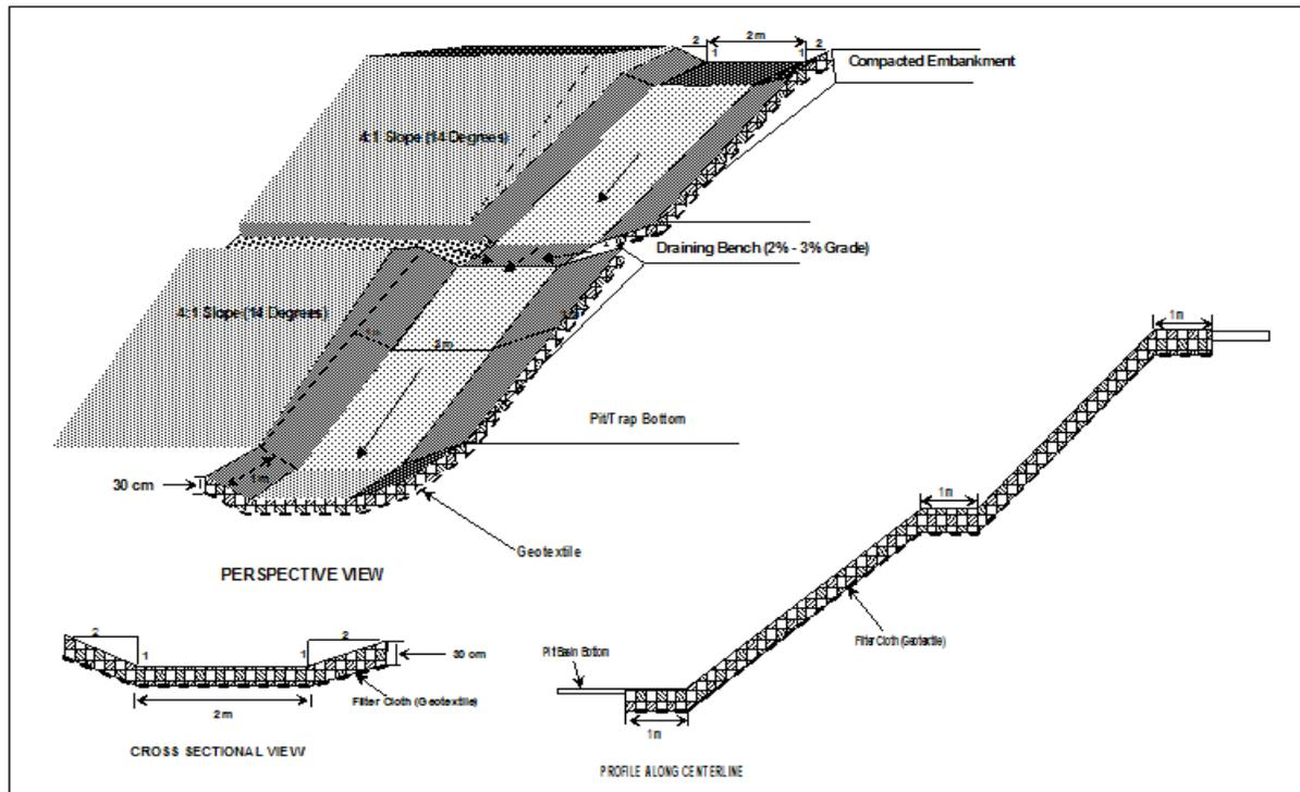
Fig. 5. Gabion Inflow protection details: not to scale
