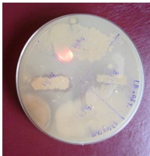
Fig.1. growth of bacillus subtilis on a LB plate supplemented with 0.6% impranil with a zone of clearing around the edges of colonies showing polyurethane degradation
