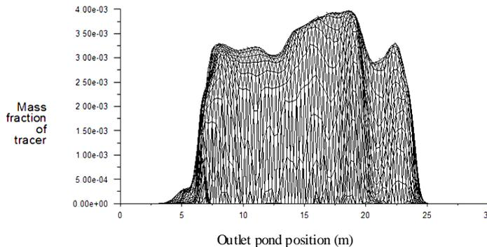
**Fig. 5.** Mass fraction tracer as a function of the outlet position in the equalization lagoon after 4.5h of the application of the tracer pulse
