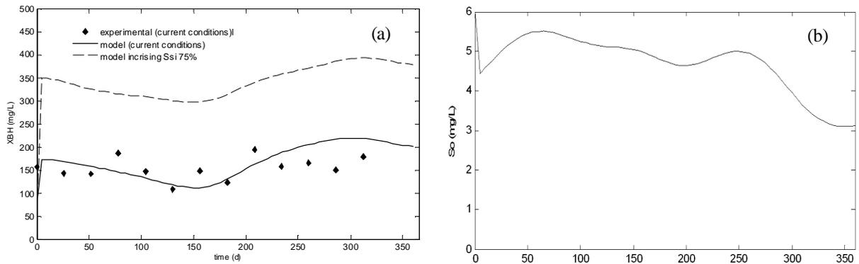
Fig. 8. Variation of (a)  $X_{BH}$  and (b) dissolved oxygen ( $S_O$ ) in the lagoon effluent, as a function of time.
