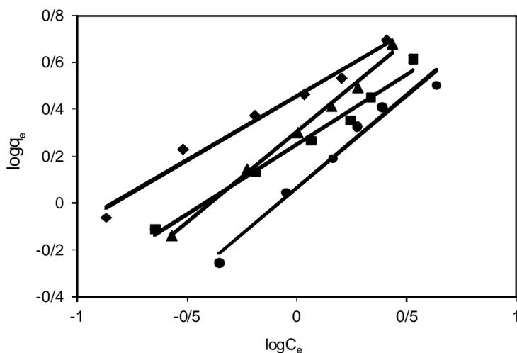
Fig. 7. Linear Freundlich isotherms of the miswak waste. (25°C, contact time 1h, pH=6, 1g/L adsorbent).
