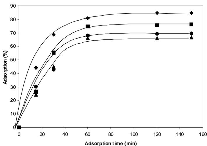
Fig. 3. Effect of contact time on the adsorption (25°C, pH=6, 1g/L adsorbent, 5 ppm initial concentration).
