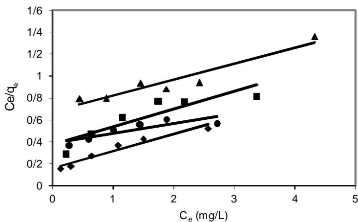
Fig. 8. Linear Langmuir isotherms of the miswak waste. (25°C, contact time 1h, pH=6, 1g/L adsorbent).
