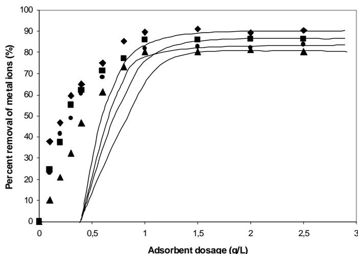
**Fig. 5. Effect of the miswak waste dosage on the removal of heavy metals (25°C, pH=6, contact time 1h, 5 ppm initial concentrations). Ni(II) ▲; Cu(II) ●; Cd(II) ■; Pb(II) ◆.**
