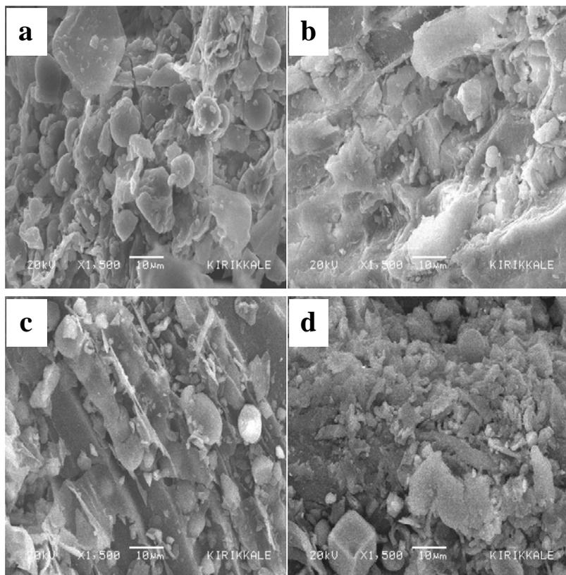
**Fig. 2. SEM micrographs of miswak waste. a. Untreated, b. Hot water-treated, c. Ethanol-treated, d. Hexane-treated**
