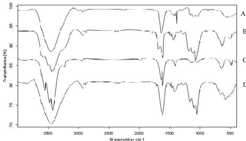
**Fig. 1. The FTIR spectrums of the miswak waste. Untreated (A), hot water-treated (B), ethanol-treated (C), hexane-treated (D)**
