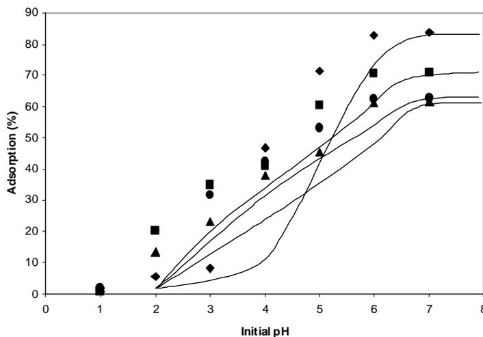
Fig. 4. Effect of pH on the adsorption (25°C, contact time 1h, 1g/L adsorbent, 5 ppm initial concentration).
