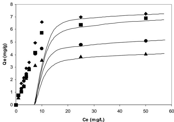
**Fig. 6. Adsorption capacities of the miswak waste. (25°C, contact time 1h, pH=6, 1g/L adsorbent). Ni(II) ▲; Cu(II) ●; Cd(II) ■; Pb(II) ◆.**
