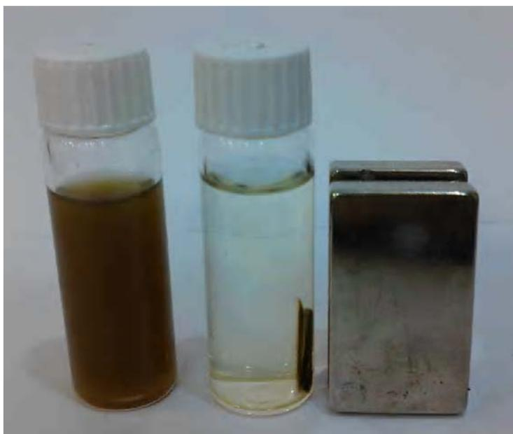
**Fig.10. BTC-Fe<sub>3</sub>O<sub>4</sub>@SiO<sub>2</sub> responded to an external magnet****CONCLUSION**
