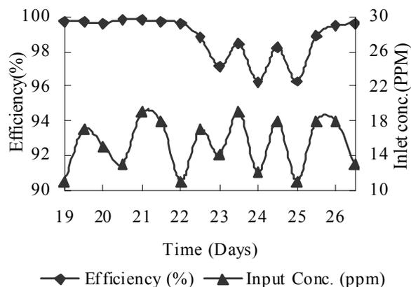
Fig. 4. Variation of H<sub>2</sub>S removal efficiency with time under third phase
