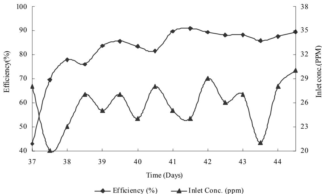
**Fig. 5. Variation of H<sub>2</sub>S removal efficiency with time under fifth phase**
