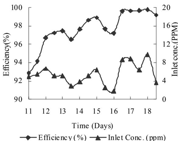
Fig. 3. Variation of H<sub>2</sub>S removal efficiency with time under second phase
