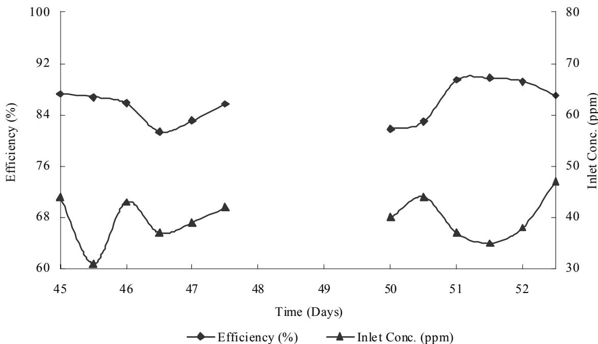
**Fig. 6. Variation of H<sub>2</sub>S removal efficiency with time under sixth phase**
