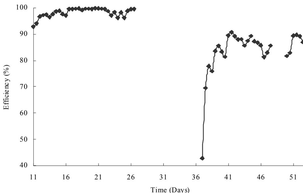
Fig. 7. Variation of Over all H<sub>2</sub>S removal efficiency with time
