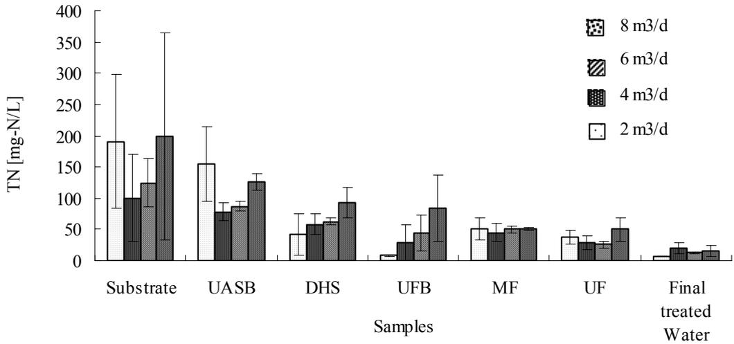
Fig. 5. Average total nitrogen removal by each process
