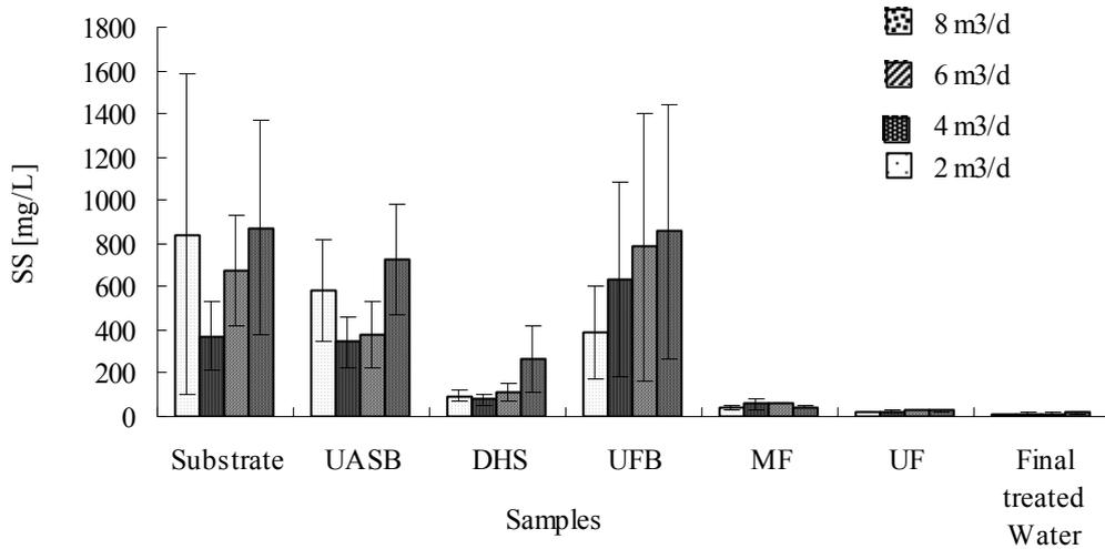
Fig. 4. Average suspended solids removal by each process
