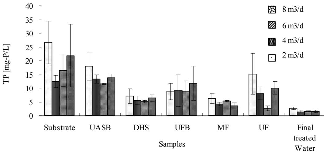
Fig. 6. Average total phosphorus removal by each process
