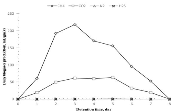
**Fig. 11. Daily biogases production at, mix ratio =1:2, pH =7.5, T =32 °C and TS =8%**
