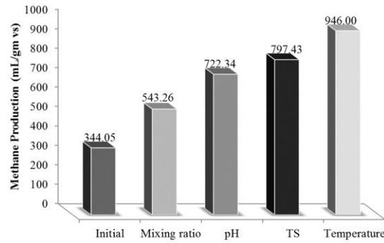
Fig. 14. Methane production increase after factors adjustment
