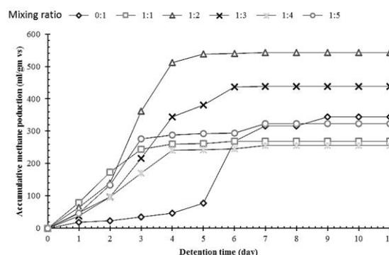
**Fig. 2. Accumulative methane production from different ratio of Algae/OFMSW at pH=7.3 and TS =10%**
