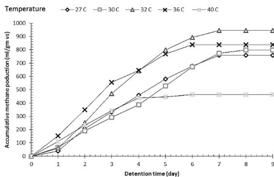
**Fig. 8. Accumulative methane production at different Temperature, mix ratio = 1:2, pH = 7.5 and TS=8%.**
