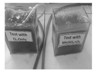
Fig. 1. Illustration of the experimental Test setup: (I) Tannery Effluent + Pure Oxygen Injection at 0.5 LPM (7 hrs duration), (II) Tannery Effluent + MnSO<sub>4</sub> addition (once) before start + Pure Oxygen Injection at 0.5 LPM (7 hrs duration)
