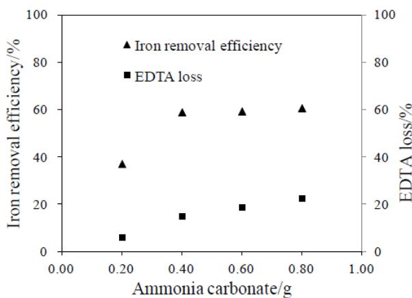
Fig. 5. Effect of the amount of ammonia carbonate on ferric ion removal efficiency
