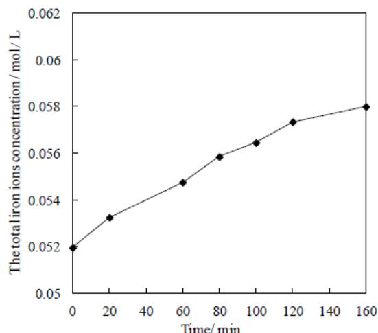
Fig. 4 .Variation of the total iron ion in the scrubbing solution
