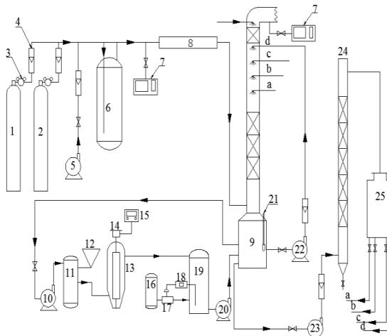
**Fig.1. Diagram of the pilot scale reactor of removing  $\text{SO}_2$  and NO**
