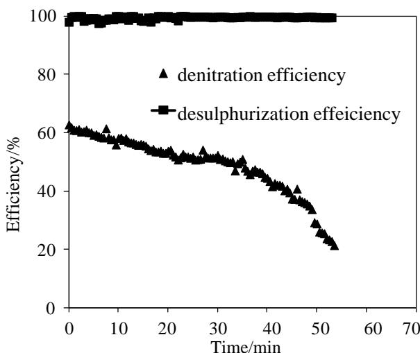
Fig.2. Ammonia/  $Fe^{II}$  EDTA desulfurization and denitration without regeneration
