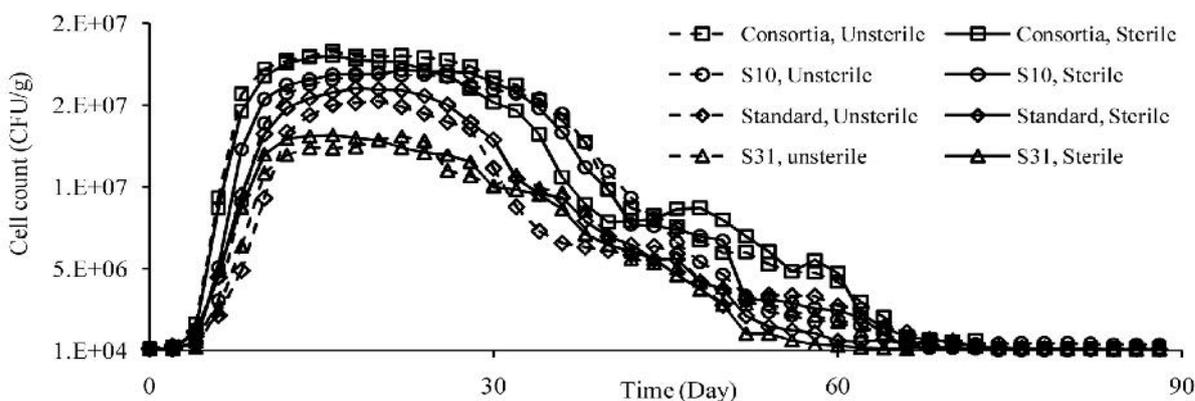
Fig. 5. Growth kinetics of standard strain,  $S_{10}$  and  $S_{31}$  isolates and their consortia in the microcosm containing enriched soil samples with 2% Karoon-3 crude oil, urea,  $KH_2PO_4$  and  $K_2HPO_4$ , under sterile and unsterile conditions, during 90 day of incubation time
