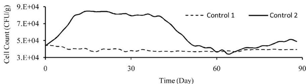
**Fig. 3.** Growth kinetics of two control samples under unsterile conditions during 90 days of incubation time. **Control 1:** The control sample containing Karoon-3 soil with aeration and moisturizing; **Control 2:** The control sample containing Karoon-3 soil with aeration, moisturizing enriched with 2% of Karoon-3 crude oil, urea and potassium phosphate. All the control samples were without any added microorganisms
