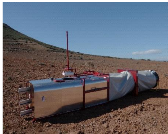
Fig. 1. Cambisol wind tunnel
