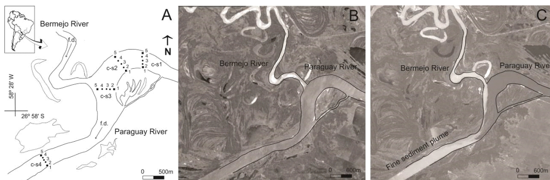
Fig. 1. Plan view of the Bermejo and Paraguay Rivers confluence. A, location of sampling cross-sections and stations (2 to 4 = sampling stations located at the central strip; 1 and 5 = bank stations). B and C, satellite images showing the sediment-laden Bermejo fluid within the less-dense water of the Paraguay River during low water stage (October 2007) and flooding, respectively. Note the increased plume of sediments in C.
