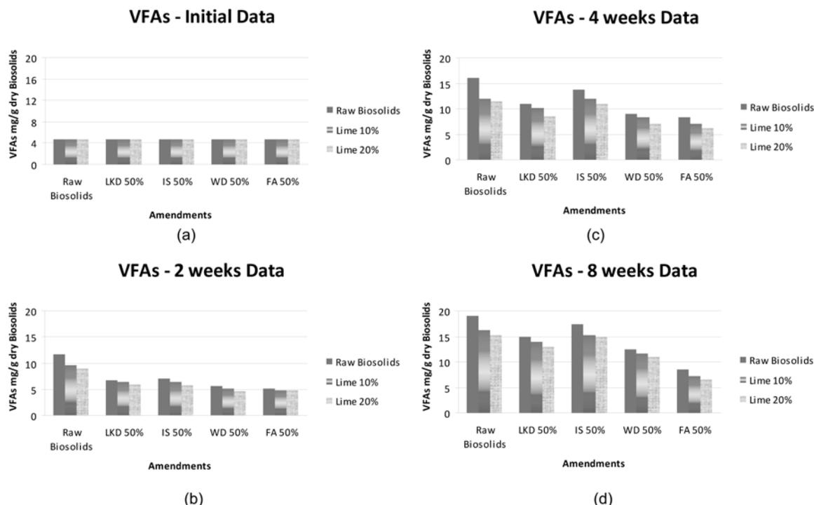
Fig. 3. VFAs increment in raw biosolids, LKD 50%, FA 50%, WD 50% and IS 50%
