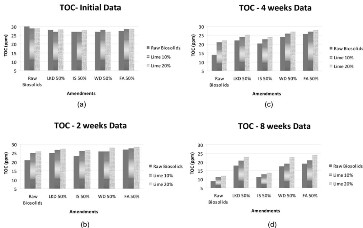
**Fig. 1. TOC degradation in raw biosolids LKD 50%, FA 50%, WD 50% and IS 50%**
