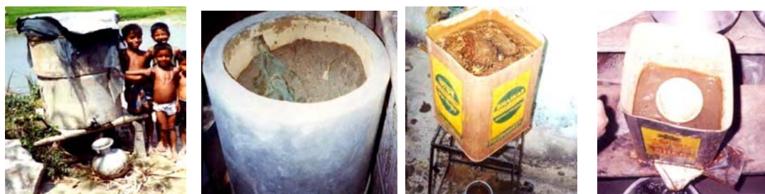
Fig. 1. Typical indigenous household iron filter units used in rural and semi-urban Assam.
