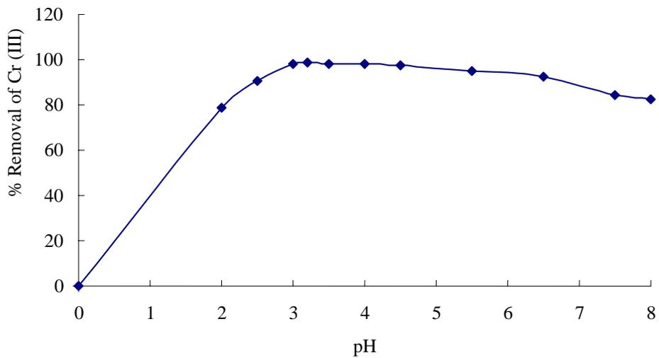
**Fig. 4. Effect of pH Cr (III) removal**
