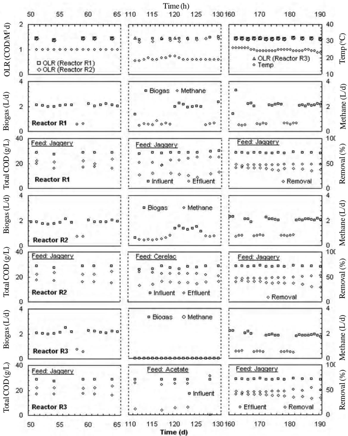
Fig. 3. Spatial variations in selected steady response of reactor R1, R2 and R3
