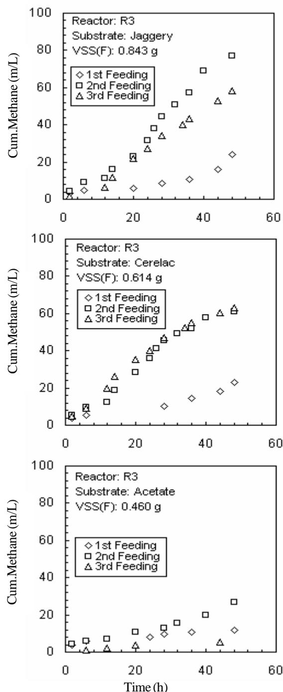
Fig. 4. Typical activity test results with reactor R3 biomass withdrawn on 116<sup>th</sup> d of operation in Phase-II
