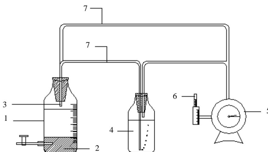
1. Aspirator Bottle 2. Anaerobic Biomass 3. Gas Outlet 4. KOH Trap 5. Gas Flow Meter 6. Thermometer
