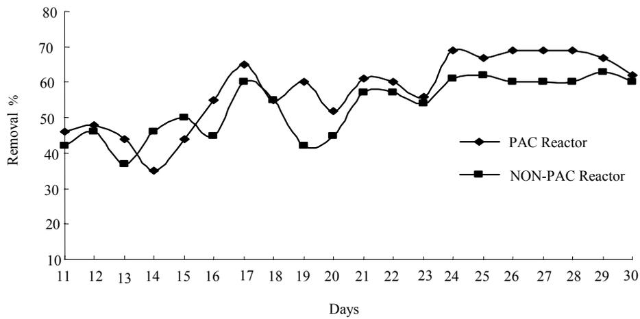
**Fig. 5. NH<sub>4</sub>-N Removal in PAC and NON-PAC reactors**
