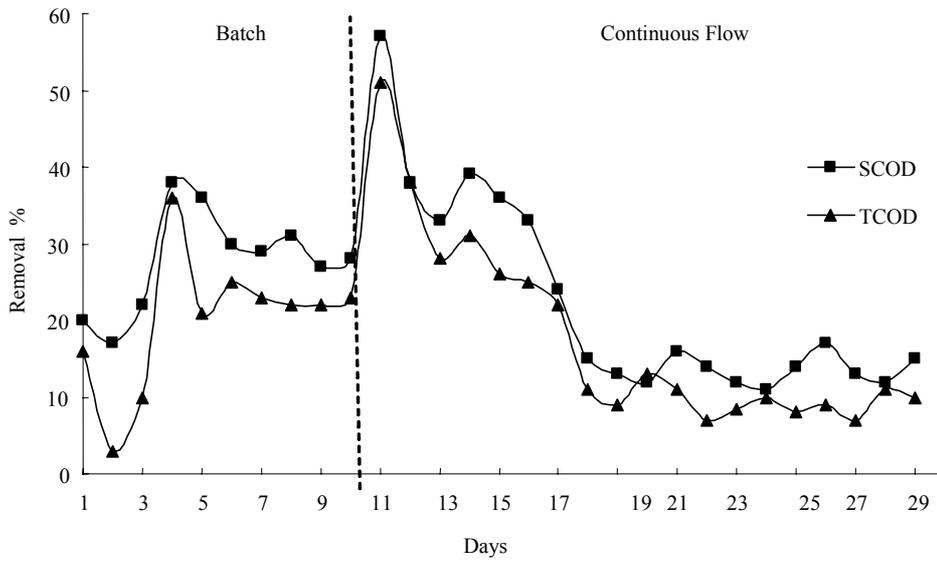
Fig. 4. COD removal efficiency in PAC reactor
