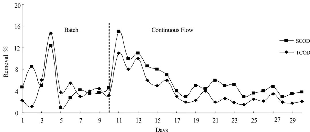
Fig. 3. COD removal efficiency in NON-PAC reactor
