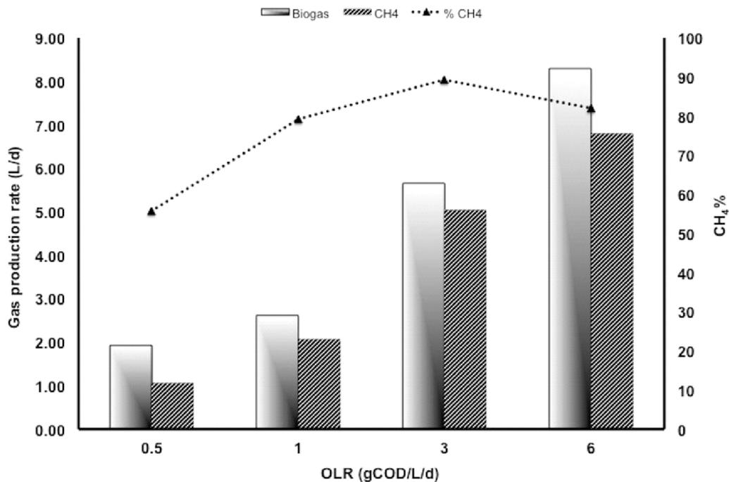
Fig. 3. CH<sub>4</sub> and %CH<sub>4</sub> biogas production versus OLR
