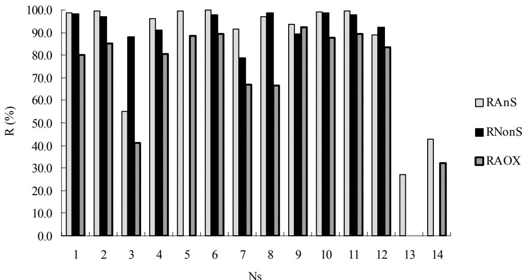
Fig. 2. Removal efficiencies of surfactants ( $R_{AnS}$  and  $R_{NonS}$ ) and AOX ( $R_{AOX}$ )
